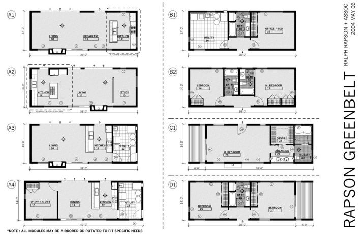
Figure 5. Internal document produced by Ralph Rapson and Associates illustrating module component variations to further customize the Greenbelt house types
